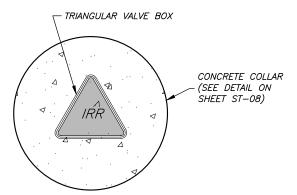
STREET VALVE COVER NOTE: LID FOR SECONDARY WATER TO BE "D&L SUPPLY" M-9009, (OR EQUAL) STAMPED "IRR" OR " IRRIGATION"
