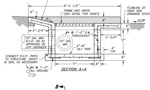
WHERE DRAINAGE ENTERS STRUCTURE FROM BOTH DIRECTIONS, FLATTEN INLET
